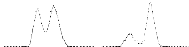
Fig. 5. Splitting of the \omega - 2\theta scan profiles observed in the LT phase of TMSO. In the left profile, the intensities of the two peaks are almost the same; in the sample used for the data collection (right profile), a clear difference is observed between the components.
